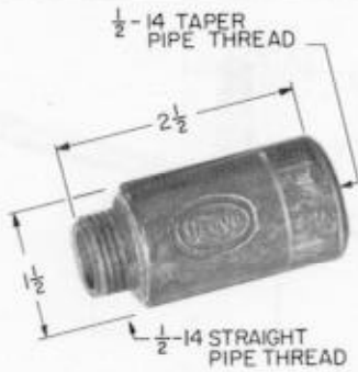
35-69 Heat Insulator. Reduces conduction of heat from sight pipe to scanner. Used with 48PT1, 48PT2, UV-1. 1/2" pipe connection.
