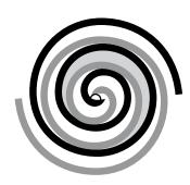
As the spiral continues to orbit, the gas is compressed into two increasingly smaller pockets.
