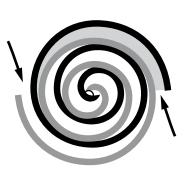
Compression in the scroll is created by the interaction of an orbiting spiral and a stationary spiral. Gas enters the outer openings as one of the spirals orbits.
