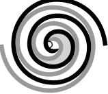
By the time the gas arrives at the center port, discharge pressure has been reached.
