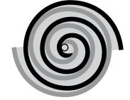
Actually, during operation, all six gas passages are in various stages of compression at all times, resulting in nearly continuous suction and discharge.
