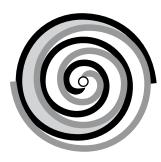
The open passages are sealed off as gas is drawn into the spiral.
