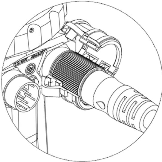
To install lockout device, place around cordset end with arrow facing the device and close until connector snaps closed.
