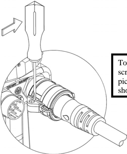
To remove lockout device, insert small screwdriver into locking groove as shown in picture. Rotate screwdriver in direction shown until locking device releases.
